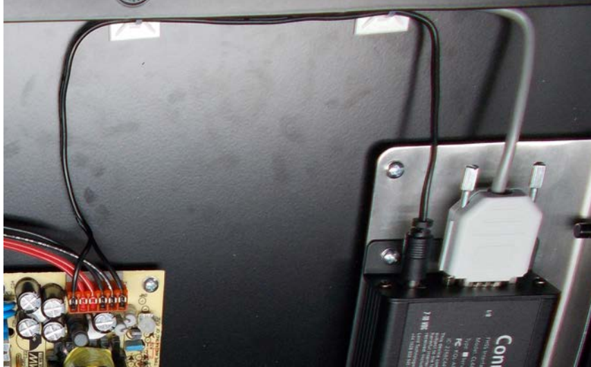
Figure 10. Connect Cable Assemblies
