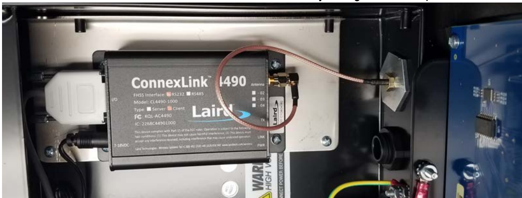
Figure 8. Mount ConnexLink Radio to Bracket
