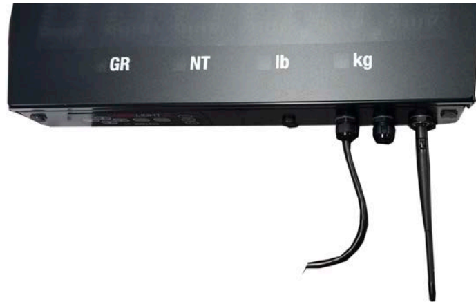
Figure 5. Thread Antenna onto LaserLight2
