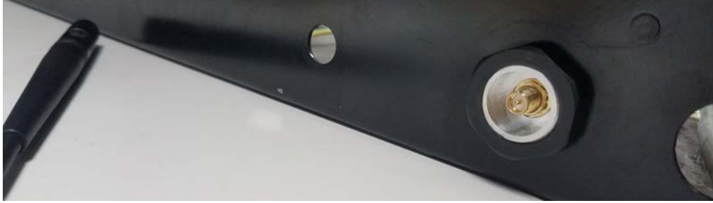
Figure 4. Thread Antenna Extension Cable Through
