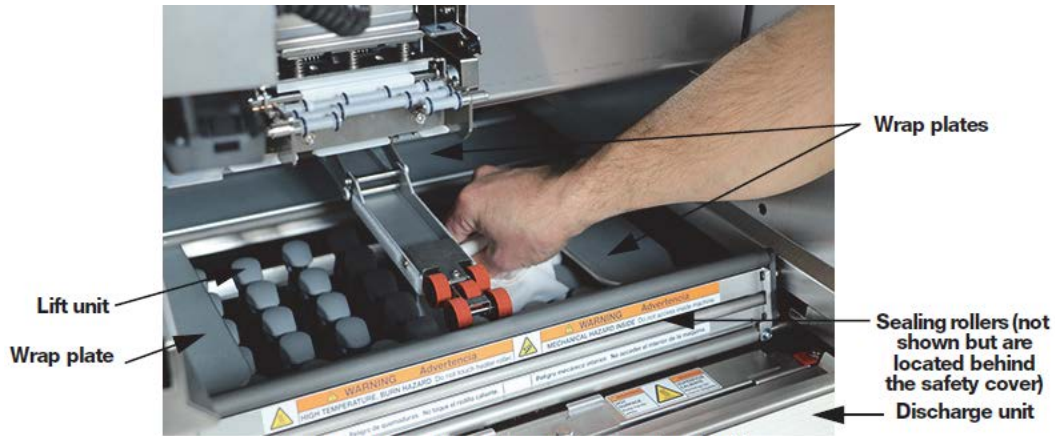
Figure 4. Clean Lift Unit, Wrap Plates and Seal Roller
