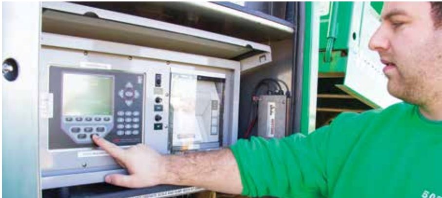
TradeRoute's 920i indicator and built-in printer provide a complete mobile weighing solution, as well as documentation for customers and management.
