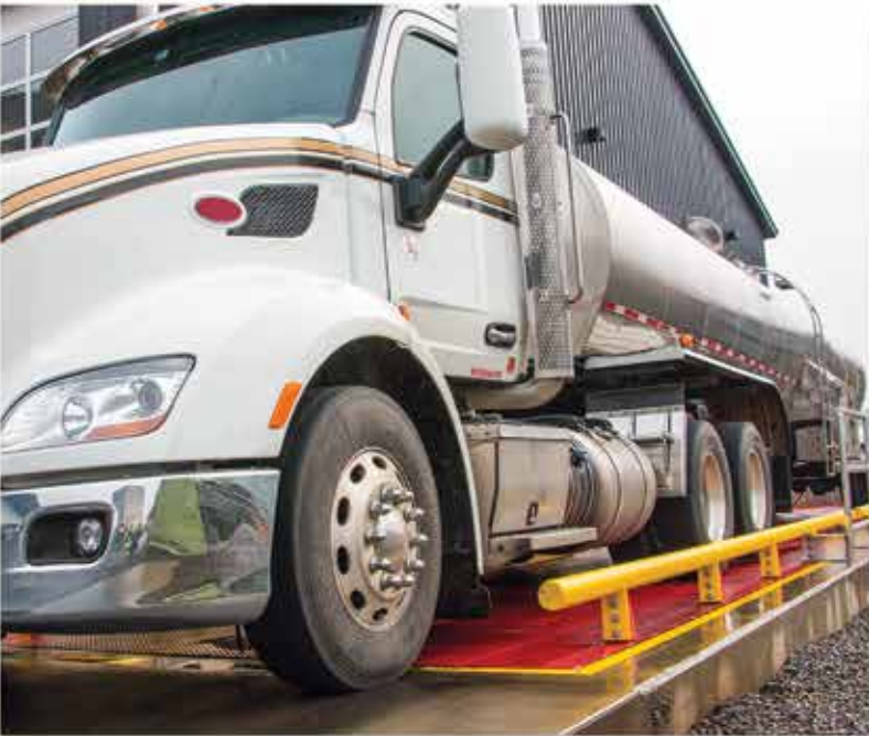
Above: A to Z Wineworks' efficiency was increased by bulk-weighing incoming shipments of wine and fruit on a SURVIVOR OTR truck scale. A tanker truck exits the scale after delivering a shipment of wine.
