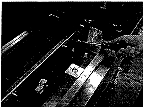
1. Remove the weighing conveyor.
