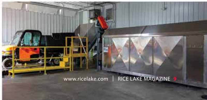
The custom RoughDeck floor scale weighs a utility vehicle as it unloads materials into the hopper. Weighments are used to determine proper amounts of supplements necessary to expedite the composting process.
