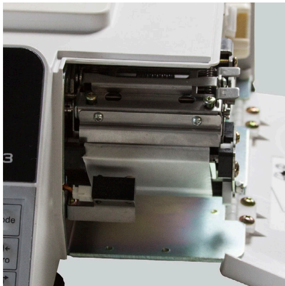
Figure 3-10. Remove Front Printer Cover
