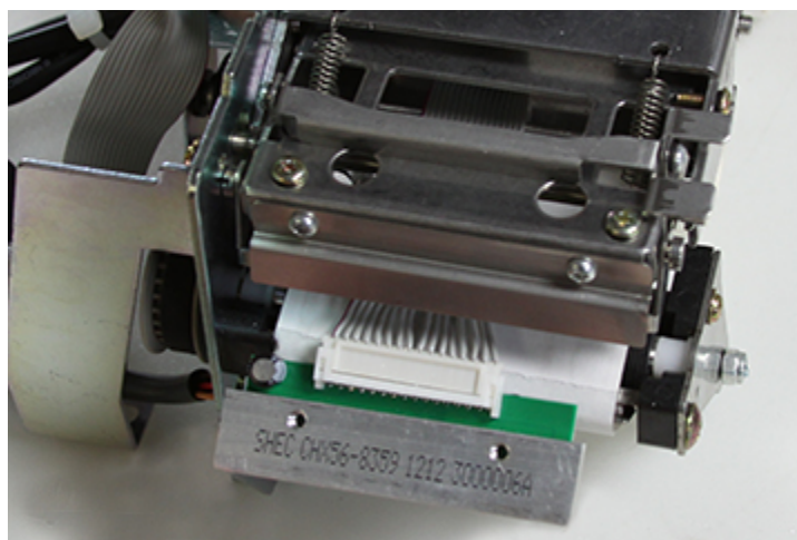
Figure 3-16. Unlatch Thermal Head Bracket
