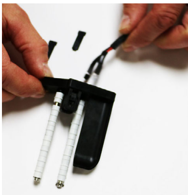
Figure 3-26. Insert Sensor Assembly
