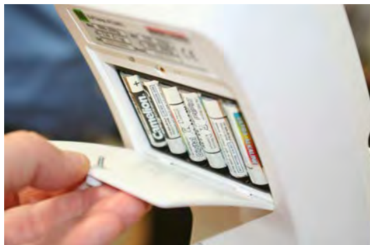
Figure 2-8. Batteries in Battery Chamber
