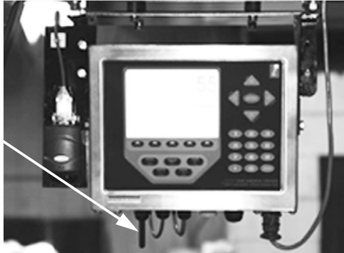
Figure 3. Location of the WLAN Antenna
