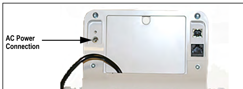
Figure 2-8. Power Connection Site
