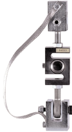
Module with RL20001HE S-beam load cell
