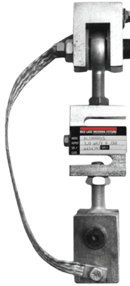
Module with RL20000I S-beam load cell
