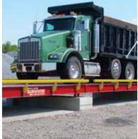
Keeping the foundation clean and welldrained will help ensure a more accurate and dependable vehicle scale.
