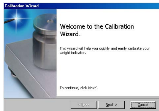
Figure 4-2. Revolution Calibration Wizard Enter the Value of Test Weight to be used for span calibration then click OK.
