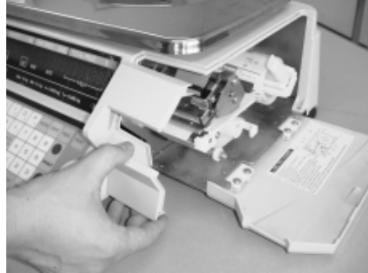
2. Remove the two screws underneath the scale and remove the front printer cover.
