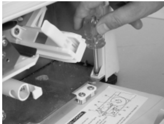
4. Remove the screw fastening the cover. Tip the cover forward.
