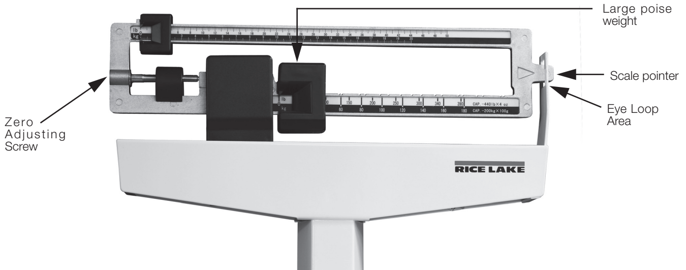
Figure 3-1. Eye Loop Area and Zero Adjusting Screw Location (Lb/Kg model shown)
