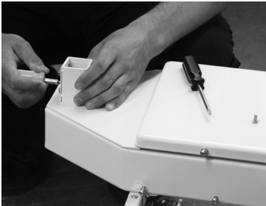
Figure 2-3. Remove Screws From Scale Base and Insert Pillar and Beam into Scale Base Assembly
