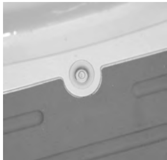
Figure 2-9. Bubble Indicates Scale Is Level
