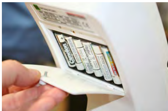
Figure 2-7. Batteries in Battery Chamber
