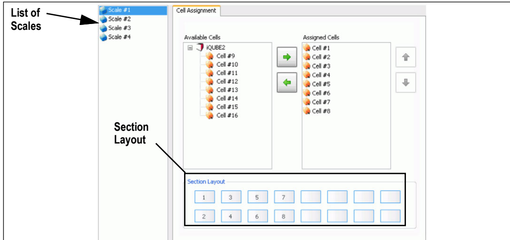
Figure 5-6. iQUBE 2 Section, Load Cell Assignment
