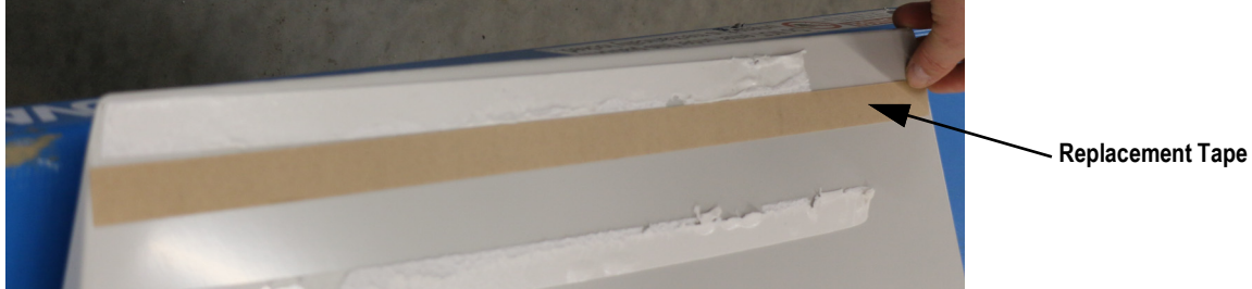
Figure 9. Double Sided Foam Tape Placement
