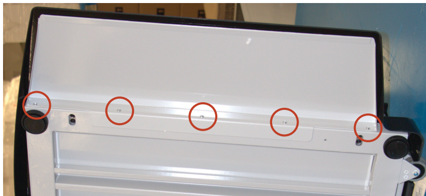
Figure 1. Ramp Screw Locations
