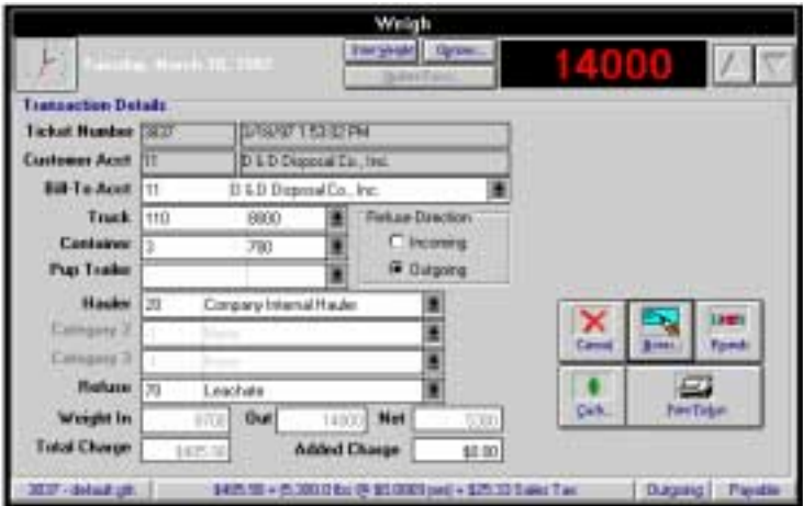
Tare Weight Applied to Outgoing Material Leaving a Site
