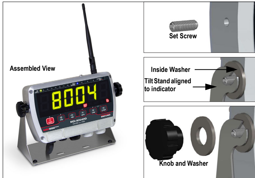
Figure 2-9. Install Tilt Stand
