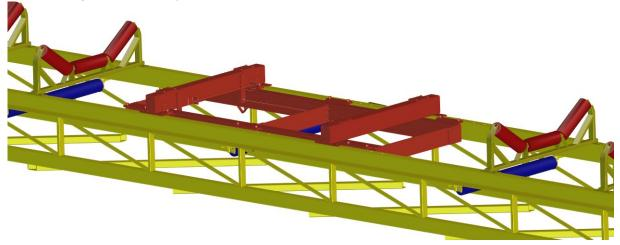
Figure 2-3. Add Weigh Frame Assembly to Conveyor
