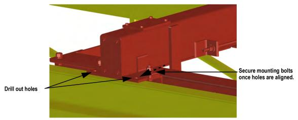
Figure 2-6. Use Bolts to Position Weldment
