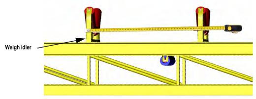
Figure 2-1. Measure Center-to-Center Distance of the Idlers
