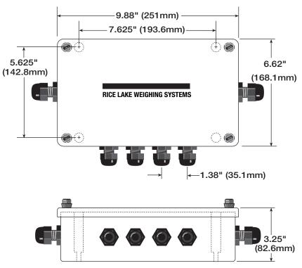
Figure 2-1. EL304A Enclosure Dimensions
