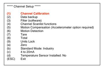
2) Start the Calibration procedure by pressing 1.
