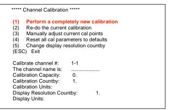
4) The MSI-9000 CellScale prompts for the calibration units of mass. Press **number** value corresponding to desired units.
