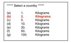
This list is for a type 'A' scale with up to 10000 counts resolution. This is the standard default. MSI recommends all MSI-6260CS Series crane scales calibrated at 5000 divisions or less. Too many divisions will compromise stability and settling time. Use the largest division size suitable for your application.
