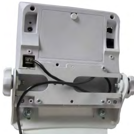
Figure 2-9. Ensure Load Cell Cable Does Not Get Pinched Prior to Putting Back Cover On
