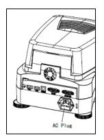
Connect the power cord to the power supply socket located at the rear of the Moisture Analyzer and to the power supply outlet. The Moisture Analyzer becomes operational as soon as power is applied. The display will remain off until the **On/Off** button is pressed.
