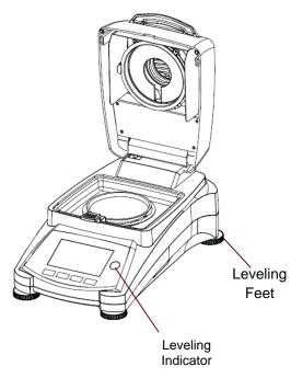
Adjust the leveling feet of the Moisture Analyzer until the air bubble in the indicator is centered. The level indicator is located under the cover towards the rear of the Moisture Analyzer.
