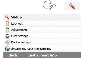
Press Setup button to access the Setup menu.
