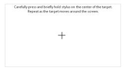
Press **Touch screen adjustment** to adjust the touch screen. Press the **Start** button to start the adjustment.
