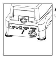
**Attention:** The RS232 port (COM 1) is located near the USB device port.
