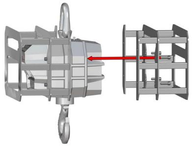
Figure 2-4. Install Back Weldment.
