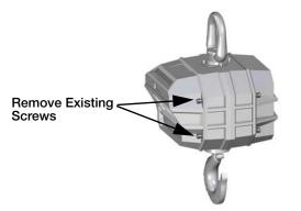
Figure 2-1. Remove Existing Screws
