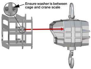
Figure 2-3. Assemble Front Cage Weldment to Crane Scale
