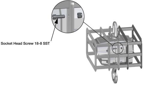
Figure 2-5. Secure Cage Weldments
