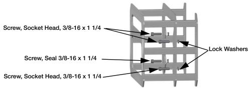
Figure 2-2. Hardware in Front Cage Weldment
