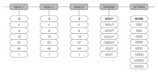
Figure 7-3. Digital Filtering Parameters on the Configuration (CONFIG) Menu
