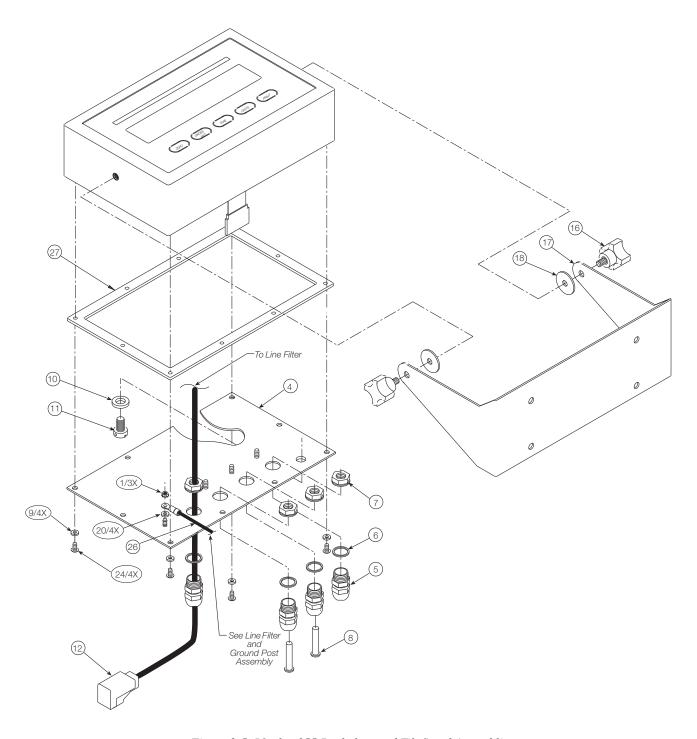
Figure 2-5. IQ plus 355 Backplate and Tilt Stand Assemblies
