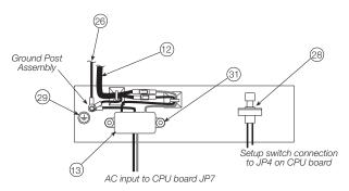
Figure 2-7. Line Filter Assembly
