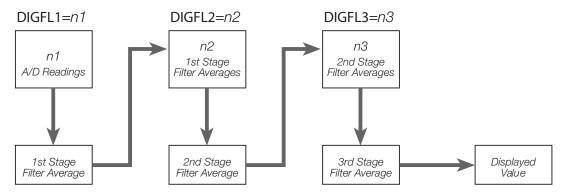
Figure 7-4. Flow Diagram for IQ plus 355 Digital Filters
