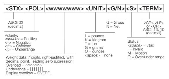
Figure 7-1. Continuous Output Data Format
