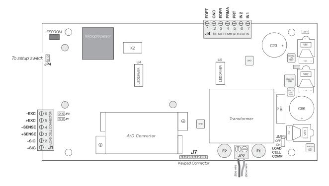
Figure 2-3. IQ plus 355 CPU and Power Supply Board
