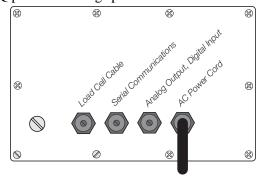
Figure 2-1. Recommended Cord Grip Assignments
