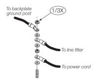
Figure 2-8. Ground Post Assembly
