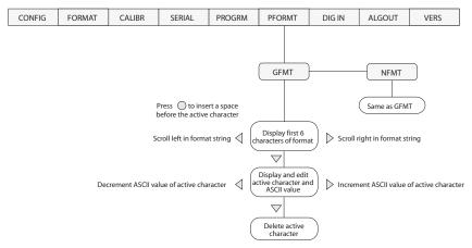
Figure 5-1. PFORMT Menu, Showing Alphanumeric Character Entry Procedure
