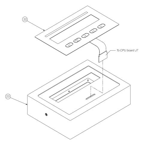
Figure 2-9. IQ plus 355 Enclosure and Overlay
