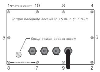
Figure 2-4. IQ plus 355 Enclosure Backplate
