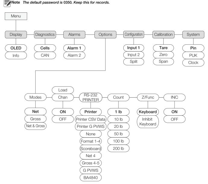
Figure 4-1. User and Setup Menu – Electrical Wiring and Data Connections
