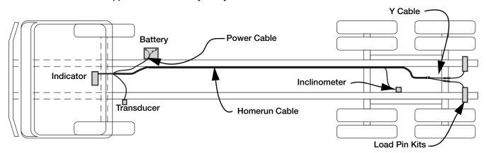
Figure 3-1. LoadRunner System Layout
