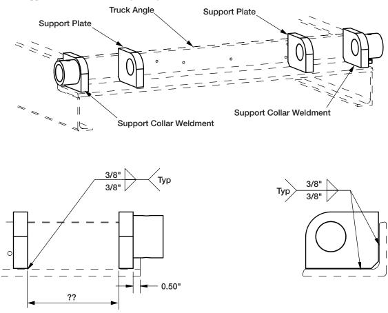
Figure 3-2. Weld Supports to Frame
