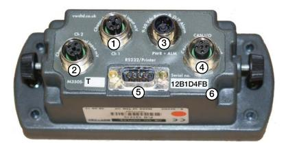
Figure 3-10. Rear Panel Identification and Bulkhead Connectors
