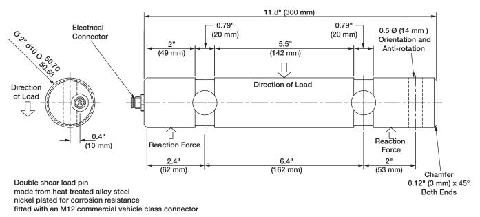
Figure 2-2. 2 Inch Diameter Load Pin (PN 131207)
