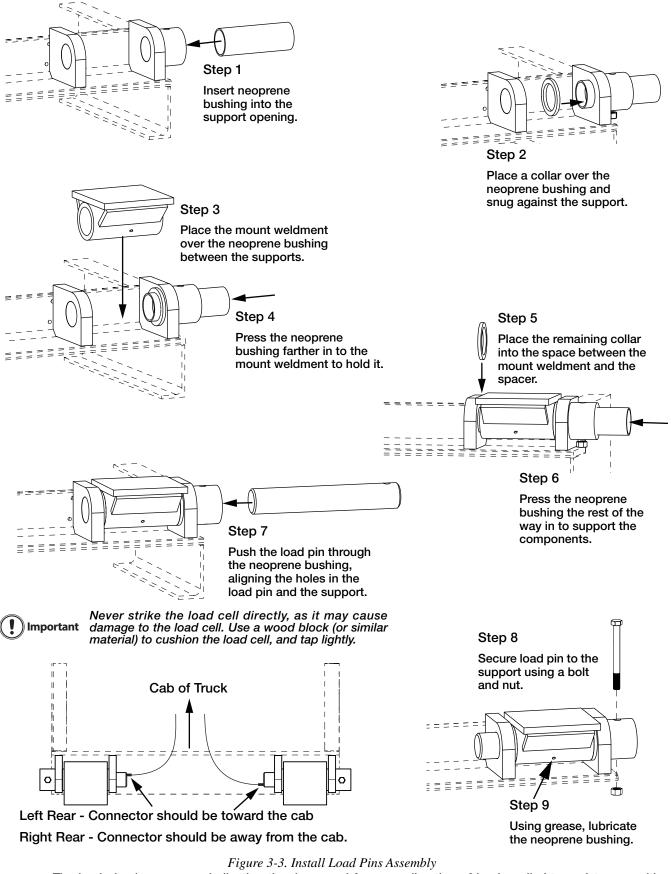
Note The load pins have arrows indicating the downward force, or direction of load applied to register a positive weight value. See Figure 2-2 for load pin specifications and load direction.
