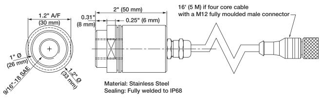
Figure 2-3. Oil Pressure Transducer (PN 131211)
