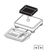
Tare the scale. This is not required if the automatic tare function is active. The tare weight is saved automatically when you place the container on the platform.
