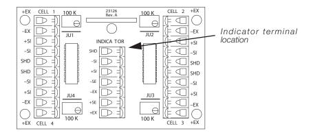
Figure 3-3. Junction Box Wiring Diagram
