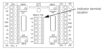
Figure 4-2. Junction Box Wiring Diagram
