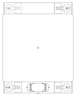
Figure 6-4. Corner Numbering - Top View of Scale
