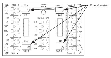
Figure 5-1. Summing Board Diagram
