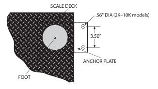
Figure 3-1. Anchor Plate Installation
