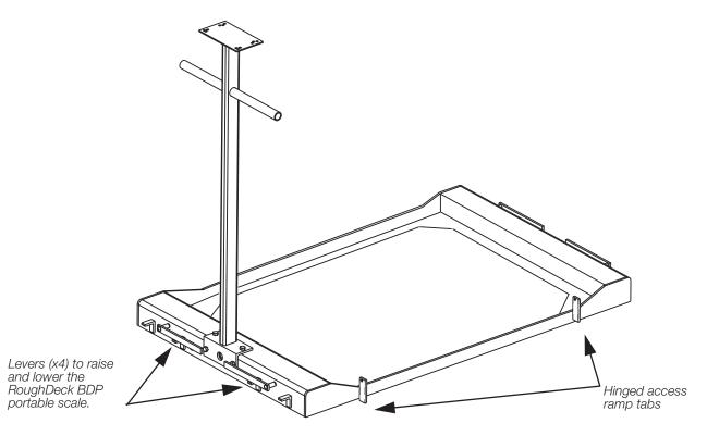
Figure 4-1. Portability Frame Kit Diagram
