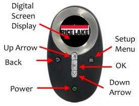
Figure 3-1. Handheld Controller Key Functions
