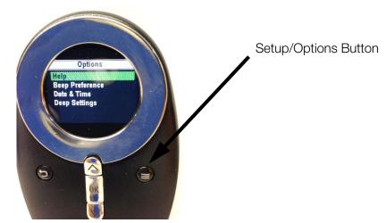
Figure 4-3. Setup/Options Button Location
