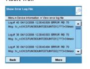
Logs important changes to the balance, so any errors or other non-conforming items can be quickly traced to the source.
