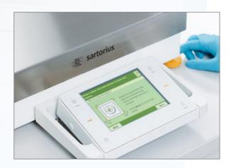
Cubis® continuously monitors whether it is perfectly level. Quick manual leveling takes just a few steps with interactive operator guidance prompts shown on the display.
