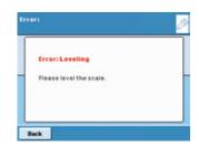
Cubis® has warning and reminder functions in combination with a configurable action hierarchy for leveling, determining the USP Chapter 41 starting point of the operating range, and for calibration | adjustment.
