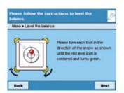
Q-Level enables you to have your balance automatically leveled by motors at the touch of a key. In the process, the Cubis® balance checks whether it is perfectly level and will immediately alert you whenever it has to be re-leveled (automatic messaging only on models with a capacity of  $\leq$  6.2 kg and a readability of > 0.001 mg).
