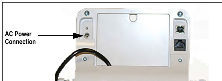
Figure 2-6. Power Connection Site
