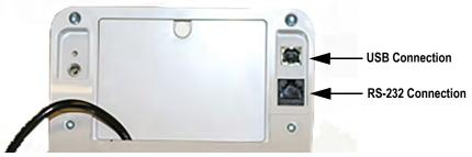
Figure 4-1. Connection Ports
