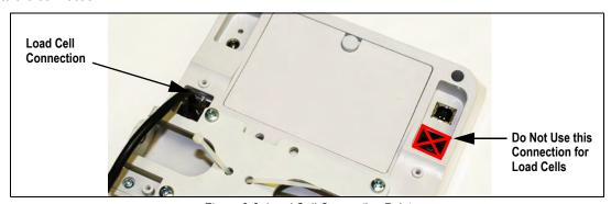
Figure 2-8. Load Cell Connection Point
