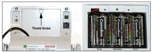
Figure 2-4. Battery Chamber
