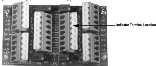
Figure 2-2. Junction Box Wiring
