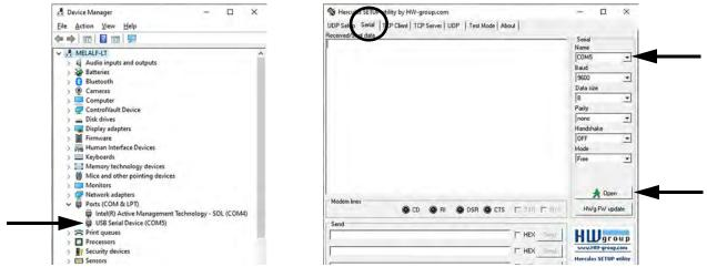
Figure 4-2. Connecting to a Serial Port
