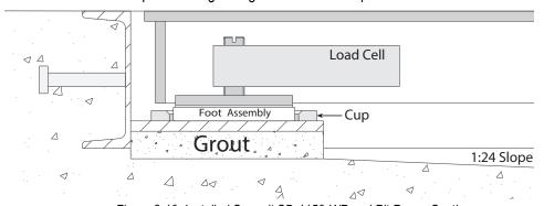
Figure 2-10. Installed Summit SD-1150-WP and Pit Frame Section
