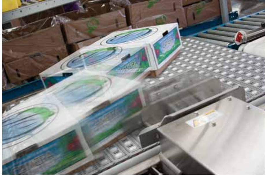
You shall not pass! MotoWeigh's diverter sends overweight and underweight boxes to a reject line.
