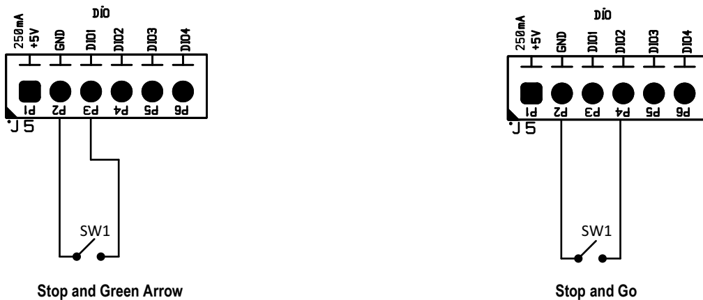
Figure 4-23. Single Switch DIO Wiring
