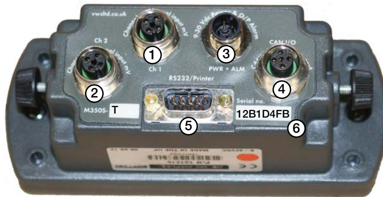
Figure 3-3. Rear Panel Identification and Bulkhead Connectors
