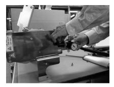
3. Hook the AD-4982 onto the frame.
