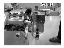
4. Using the four screws (M6X15 hex bolt) provided, secure the AD-4982 to the frame.
