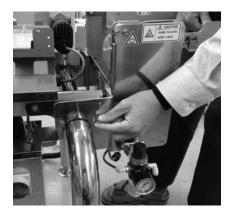
5. Confirm that the AD-4961 motor input cable does not touch the AD-4982.
