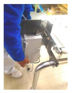
Secure the pusher module to the main unit with the provided screws (4pcs).
