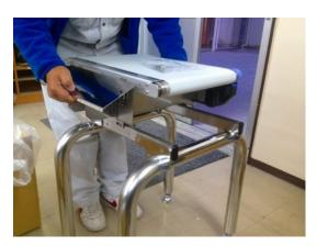
Secure the conveyor unit to the frame with the provided screws (4pcs).
