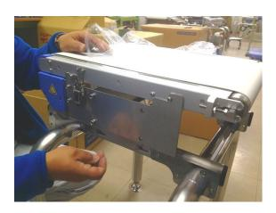
Install the pusher module to the main unit.
