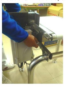
Attach the regulator to underneath the pusher module. Install an air tube to the regulator.
