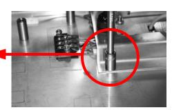
Figure 5-10. Secure Heater to Enclosure Bottom
