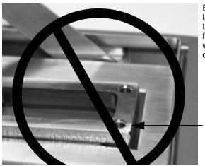
Ensure that the larger side of the tapered pocket is facing upwards when placing it on the four studs
