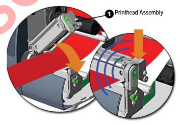
Figure 1-24. Latch Printhead Assembly
