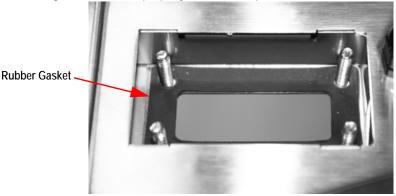
Figure 1-7. Rubber Gasket
