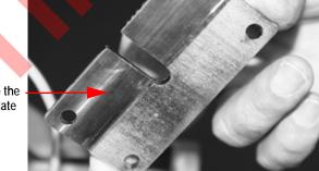
Clamp plate - note the step for the half plate
