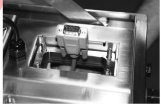
Figure 1-9. Communications Cable Comes Up Through Bottom of Hole
