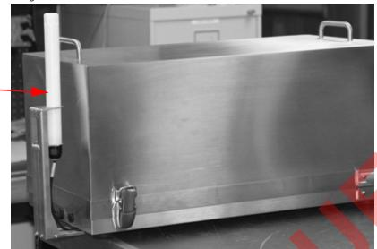
Figure 5-41. Installed Wireless Antenna
