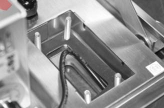
Figure 5-31. Press Down Rubber Gasket Around Bolts
