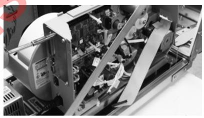
Figure 3-4. Remove Front Panel Screws
