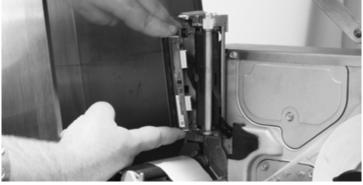
Figure 3-2. Remove Old Printhead Assembly
