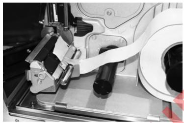
Figure 1-27. Load Printer With Media
