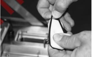
Figure 5-33. Assemble The Split Seal Plates Together
