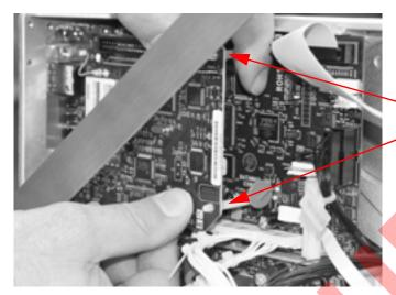
Figure 5-23. Align Communication Card to Installed Standoffs
