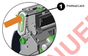
Figure 1-20. Open Printhead Latch to Load Optional Ribbon
