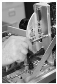
Figure 5-21. Remove Screws from Cover Plate
