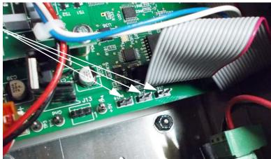
Figure 7. Locate and Remove Jumpers
