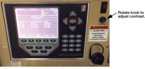
Figure 11. Contrast Control Potentiometer Installed
