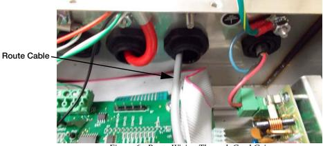
Figure 6. Route Wiring Through Cord Grip
