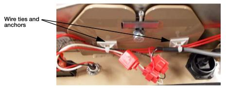
Figure 10. Secure Wires
