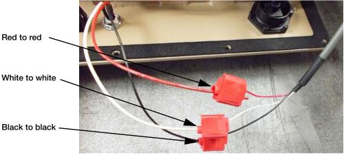
Figure 9. Connect Wires
