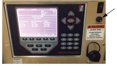
Figure 1. Contrast Control Potentiometer Installed
