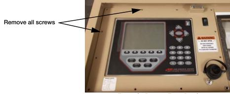
Figure 2. Remove Front Bezel
