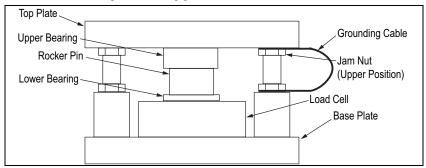
Figure 2-2. Silo Mount Assembly
