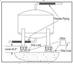
Figure 2-1. Horizontal Piping
