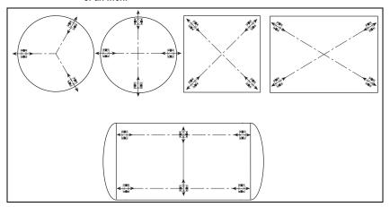
Figure 2-3. Load Cell Orientation
