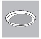
Affix the pad to the center of the sample pan, sticky side down.
