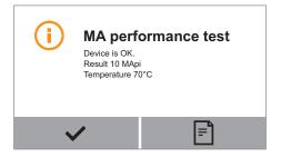
▶ If the test is successful, the message "Device is OK" first appears. Then the analyzer indicates that the sample can be removed.
