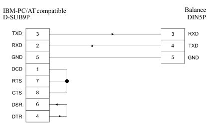
Figure 2-7. Sample connection with an IBM-PC/AT compatible
