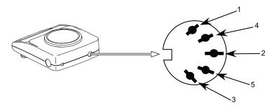
Figure 2-6. RS 232 C Connector (DIN 5-pin): Rear Panel
