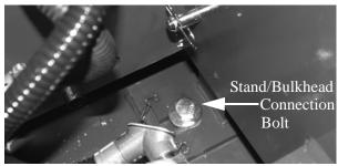
Figure 2-6. Bolt Connecting Stand to Bulkhead
