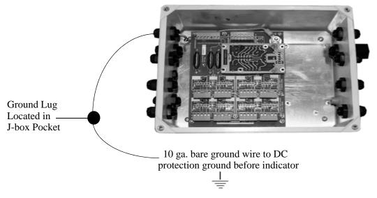
Figure 3-3. Grounding and Transient Protection on ATV Scale
