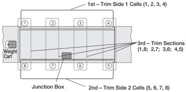
Figure 4-1. Load Cell Trimming Diagram
