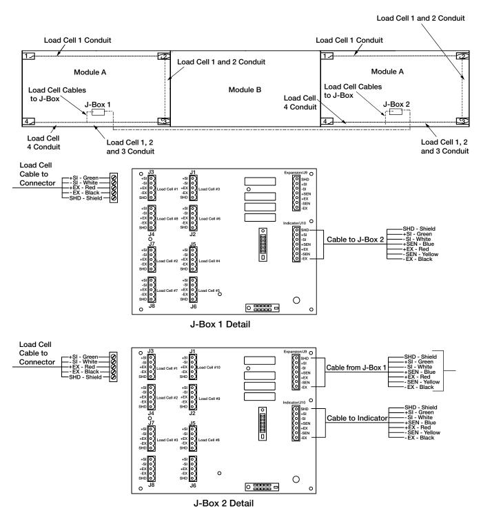
Figure 3-2. J-Box Wiring and Conduit
