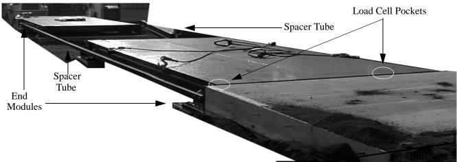
Figure 1-1. Weighbridge with Self-Contained Modules in Place
