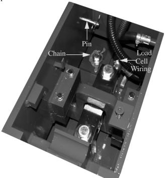
Figure 2-9. Load Cell Cover Plate Removed
