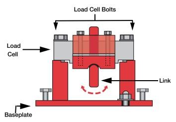
Figure 5-1. Load Cell Replacement
