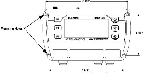
Figure 2-3. Mounting Hole Dimensions
