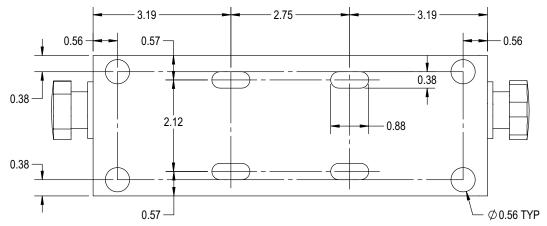
Figure 2-2. Tilt Stand – Bottom Dimensions
