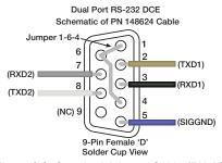
Figure 6-2. Standard Adapter Cable (PN 148624)
