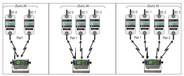
Figure 6-1. Multiple Sensor Network
