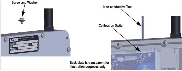
Figure 5-1. Press Configuration Switch
