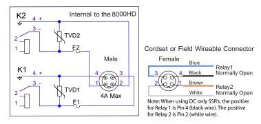
Figure 6-7. Cordset or Field Wireable Connector
