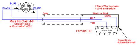
Figure 6-5. DCE Configuration for Computer Connection
