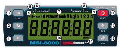
Figure 1-1. MSI-8000HD Front Panel
