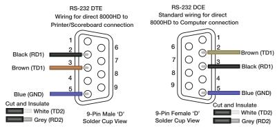
Figure 6-4. Communications Port 2 Wiring
