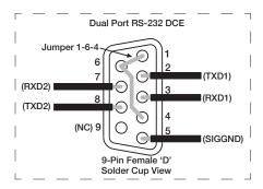
Figure 6-3. Communications Port 1 Wiring
