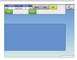
2. Available preset keys are listed on the screen. To turn pages, press [▼] or [▲]. Press a desired function for selection.
