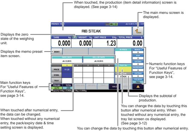
You can change the data by touching this button after numerical entry. When touched without any numerical entry, the markdown price input screen is displayed.
