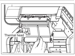
**4.** In the same way, dip the attached felt tip pen in the cleaning solution, and lightly wipe the surfaces of the print roller and auxiliary roller with the pen.
