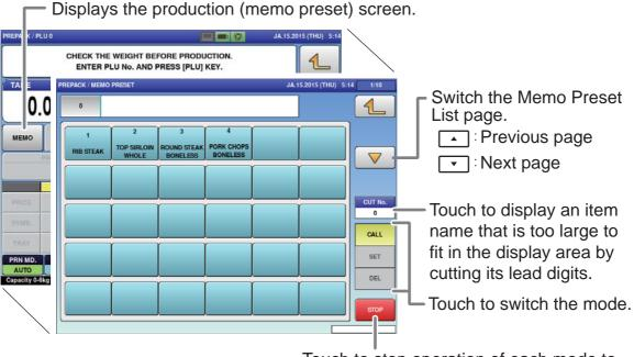
Touch to stop operation of each mode to return the display to the production screen.
