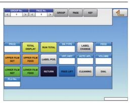
2. To create or delete the group or the page, press the [GROUP] or [PAGE] button, and then press a desired function button as shown below.
