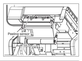
**3.** In the same way, dip the attached felt tip pen in the cleaning solution, and lightly wipe the surface of the thermal head with the pen.
