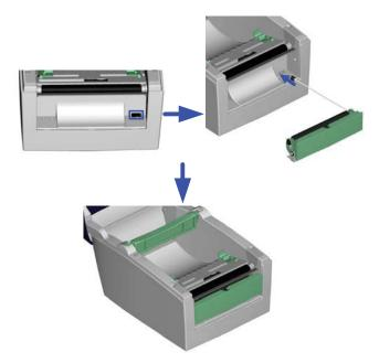
7. Turn the printer around and tighten screws to secure the stripper module.
