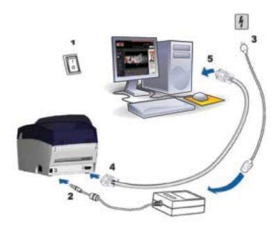
Figure 2-1. PC connection illustration
