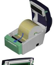
13. Feed the label through the cutter and press the FEED key to complete the installation.
