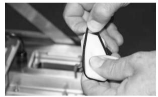
Figure 2-8. Assemble Split Seal Plates Together
