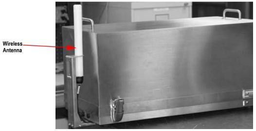
Figure 5-35. Installed Wireless Antenna
