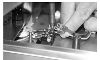
Figure 5-11. Color Match Wire Harness and Terminal Strip Wires
