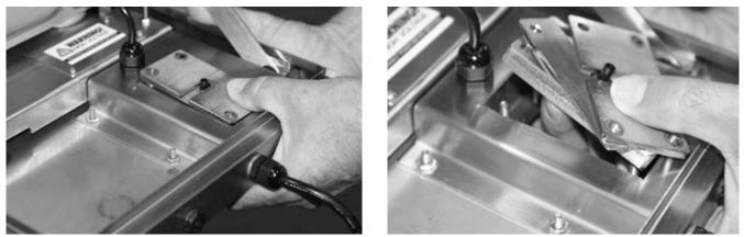
Figure 2-3. Remove the Component Parts of the Communications Cable Assembly
