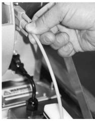
Figure 2-9. Connect Communications Cable to Back of Printer
