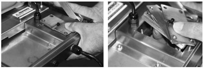
Figure 5-21. Remove the Component Parts of the Communications Cable Assembly
