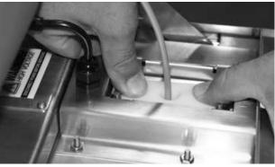
Figure 2-10. Seat the Split Seal Assembly
