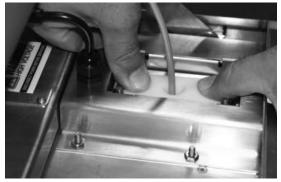
Figure 5-29. Seat the Split Seal Assembly
