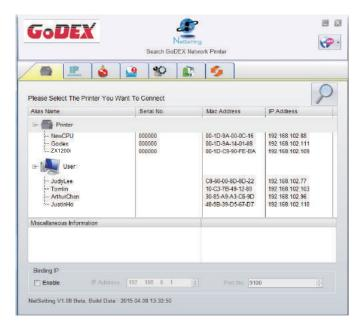
Click the magnifier icon to search the Godex printers which are connected via Ethernet port in the network environment. Once a connected Godex printer is detected, it will be listed on the start page.
