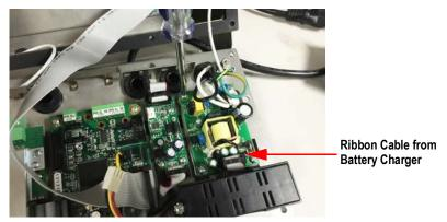
Figure 8. Reinstall Power Supply Board
