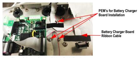
Figure 4. Battery Charger Ribbon Cable Routing
