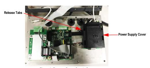
Figure 1. Remove Power Supply Cover
