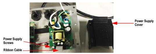
Figure 2. Loosen Power Supply Board
