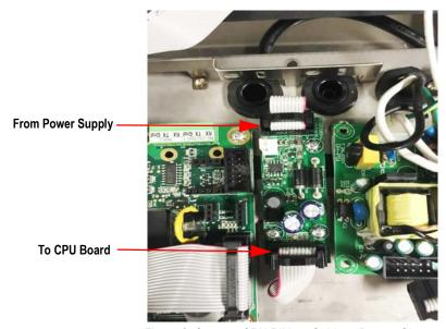
Figure 6. Connect CPU Ribbon Cable to Battery Charger
