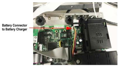
Figure 9. Battery Connector to Battery Charger Board
