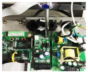
Figure 5. Install Battery Charger
