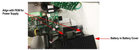
Figure 7. Install Battery
