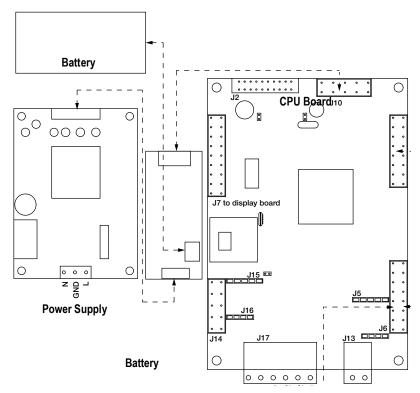
Figure 10. Wiring Diagram
