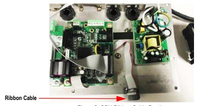
Figure 3. CPU Ribbon Cable Routing
